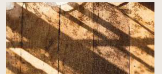
Avoid Direct sunlight / continuous light form the HPL Sheet These may cause to color fading due to UV Rays
